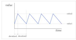
The value follows a cycle where it changes linearly from value1 to value2 during duration1 and changes from value2 to value1 during duration2.
