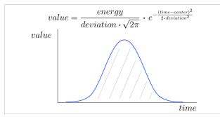
The value follows a gaussian function normalised to have always the same energy (area under the curve) regardless of the standard deviation.
