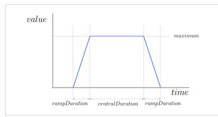
The value changes linearly from zero to maximum during rampDuration. It is equal to the maximum for centralDuration.
